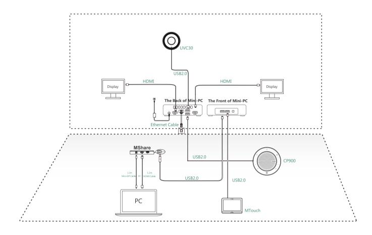
For convenience, we recommend that you connect a USB hub to the back of the Mini-PC to use mouse and keyboard to manage devices.
