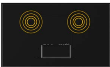
2W, 5Ω x 2 Integrated Speakers
