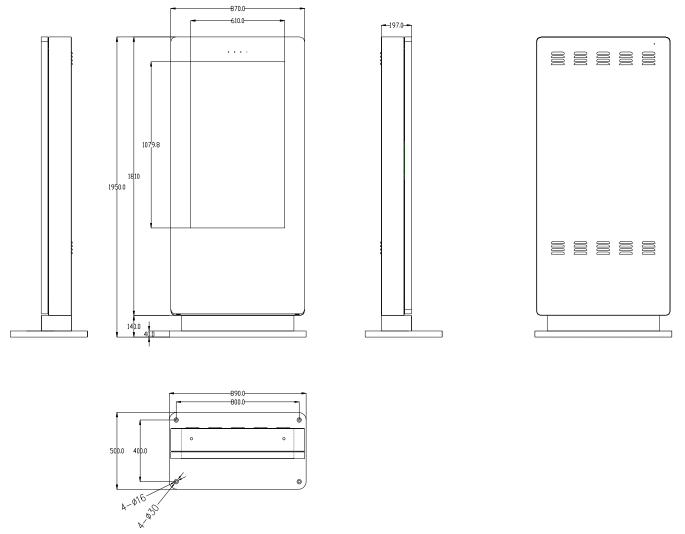
Note: The Ø30 holes are for access, we recommend using M10 anchor bolts that will fit into the Ø16 holes.
