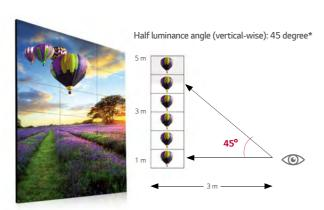
\*The angle from the center of the screen to have 50 % of the initial luminance.
